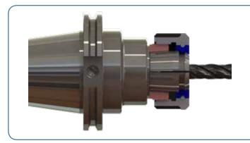
• Included 8 degree collet angle allows high precision and greater clamping torque than 16 degree ER collet chucks
